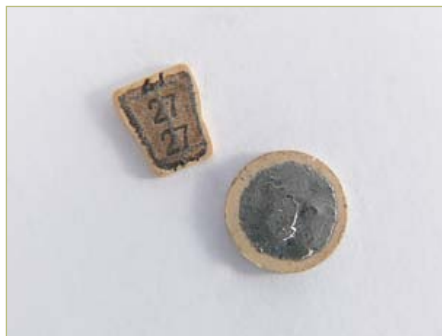
(e) Coffin and disc capacitors. Low loss factor, zero stray inductance. On-PCB coupling and decoupling. Fragile devices! Connect straight to a PCB track and copper earth plane. 27 pF, 820 pF.
