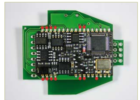
Figure 9. When fitting the DXM module only solder the indicated pins.
