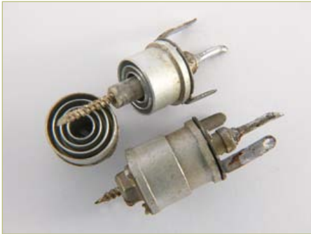
(a) Philips 'beehive' trimmers. Low loss. Ingenious construction ensures linear response across range(!) The rotor (moving part) is usually connected to ground (why?). 5–30 pF adjustable.
