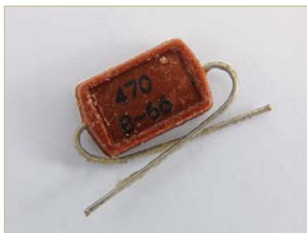
(h) Silvered mica capacitor. 500 V working voltage, 1966 NOS. Ebay-able. 470 pF.
