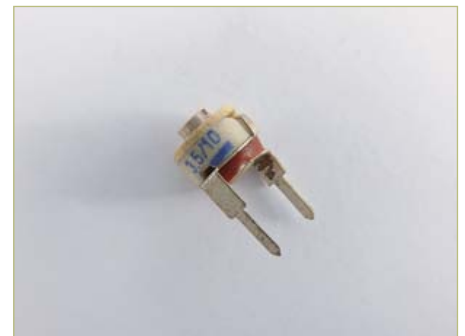
(f) Ceramic trimmer capacitor. 3.5–10 pF adjustable.
