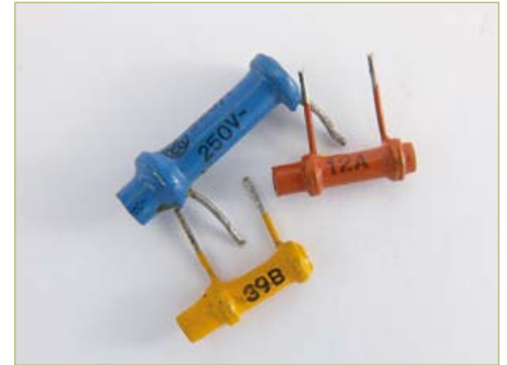
(c) Ceramic tubular capacitors. High working voltage (250 V typ.). 12 pF, 39 pF, 320 pF.
